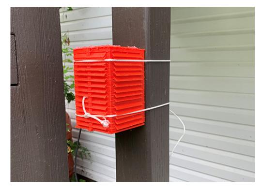
KEPO has been working with Concordia University to create an air quality monitoring network within Kahnawà:ke. Several commercial and homebuilt monitors will be set-up throughout the community to collect data on conditions year-round. KEPO will collect and analyze data from the monitors to get a picture of the overall air quality in the community.
