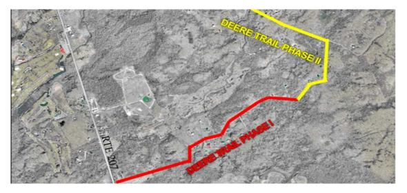
The road will be prepared to receive a two inch thick asphalt surface with the addition of a new gravel base. The gravel base will be approximately 3 inches thick. There will be minor disruptions to local traffic.
