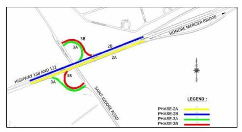
The works will be undertaken in four sub-phases (phase 2A, 2B, 3A and 3B) in an effort to localize and minimize any impacts. For more information on the sub-phases please refer to the map above.
