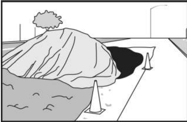
Figure 17: Impermeable Membrane Under and Over Excavated Fill
