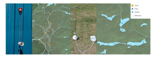
Datalogging stations in lakes have been recording the temperature and depth since they were installed in August 2022. The stations are marked by white Styrofoam buoys that are approximately 2 feet below the water's surface with reflective buoys (pictured above center) to avoid interference with boaters.
